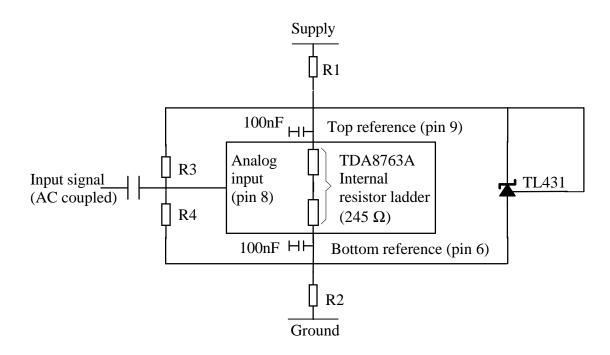
The (top - bottom) difference is set at 2.5V by the TL431, so the full scale input is set at 0.852\*2.5=2.13V. In addition the input offset is set at (Vtop+Vbottom)/2 by two equal resistors (R3 and R4).
