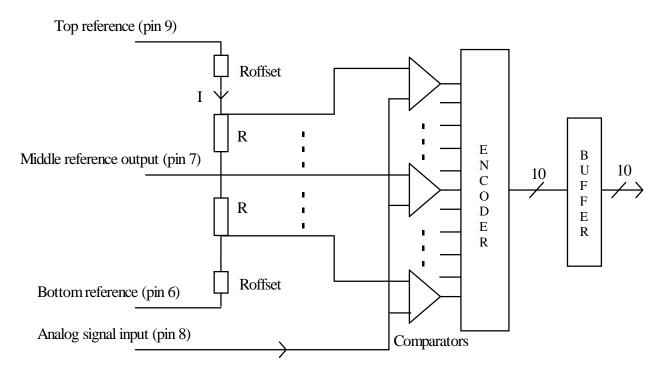
During the A to D conversion the analog input signal (pin 8) is compared to voltage references by using voltage comparators (In fact these comparators are folding amplifiers).
