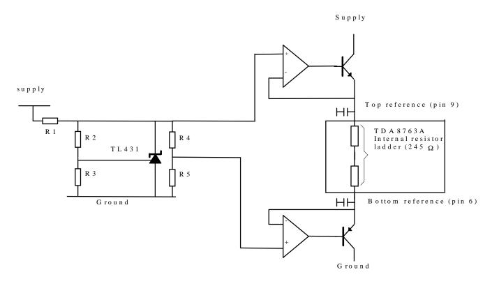
The transistor type depends on the number of TDA8763A mounted in parallel. A 9.5 mA current (typ) is required for each TDA8763A.
