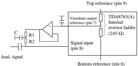
The amplifier does not need a high bandwidth, but the necessary time to load the C capacitor at 'power on' depends on the op.amp maximum output current. The input impedance is R2 // Zin. Zin is the ADC input impedance.
