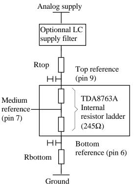
An optional filter can be added on the analog supply (depending on supply noise level).
