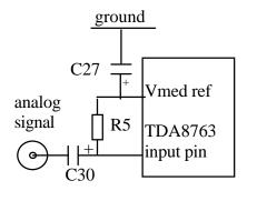
This method gives good results in the following domains: high common mode supply rejection (because both the voltage references and the input offset are derived from the same supply), very low noise level and low cost.
