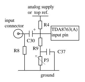
R9 is equal to the output load of the external signal generator. C37 allows ground connection between R9 and P3 in dynamic mode. Typical values when a 50  $\Omega$  signal generator is used are: R4=1K $\Omega$ , R9=50 $\Omega$ , P3=5K $\Omega$  (set at 2047 $\Omega$ ), C37=10nF, then the current flowing through the resistor bridge is only 1.2 mA with a 3.67V supply. The solder print of an optional resistor R8 is provided in order to allow other impedance adaptations
