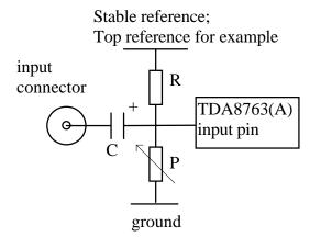
When a resistor bridge is used to provide an offset the current flowing through the resistors must be at least 10 times greater than the signal current (TDA8763(A) analog input current is 0 to 35uA) in order to guarantee the stability of the input offset. Consequently the resistive value of this resistor string must be below 10 K $\Omega$ (with a 3.67V top reference).
