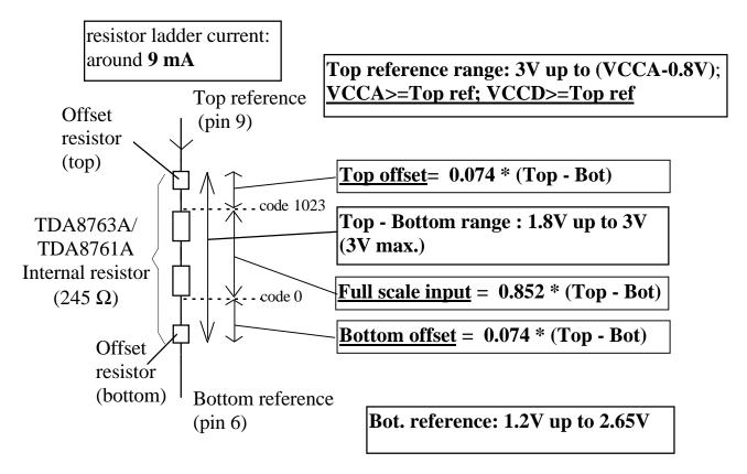
Concerning the **TDA8763**, because it has an integrated references regulator, top reference is fixed at 3.67V, bottom reference is fixed at 1.3V and the full-scale input is 2.02V. (typical values).
